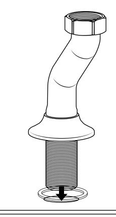
\*Remember to install the 'O' ring o washer between the mixer body & sanitary ware\*
