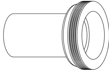
**Flushing pipe with sealing ring**
