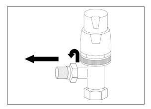
Unscrew the Compression nut and olive (clockwise) on the radiator valve and remove the provided radiator connecting spigot.
