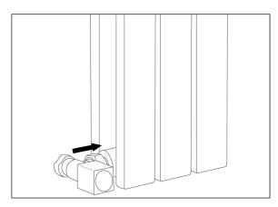
Push the circular end of the flow diverter into the radiator and screw the valve in place as normal.
