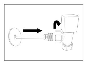
Push the fixing nut over the circular hood of the flow diverter and screw the nut anti-clockwise to secure the diverter in place.
