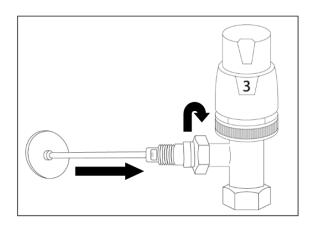
Push the compression nut and olive over the circular hood of the flow diverter and screw the nut anti-clockwise to secure the diverter in place.
