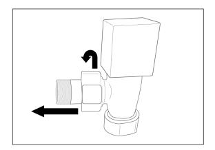
Unscrew the fixing nut (clockwise) on the radiator valve and remove the provided radiator connecting thread.
