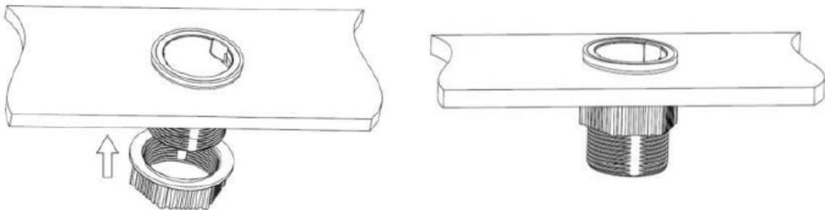
Step 4 : Insert the control body and turn clockwise to lock the control panel on the wall.
