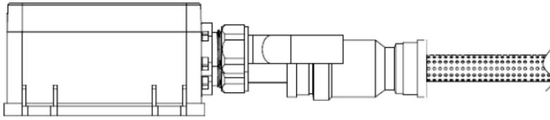
When connecting the water supplies do not apply lateral force to the inlets.
