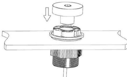
**Step 6** : Attach the control and display panel to the communication cable coming from the wall or shower panel. *Remember to put the red o-rings on any female connectors before connecting.*
