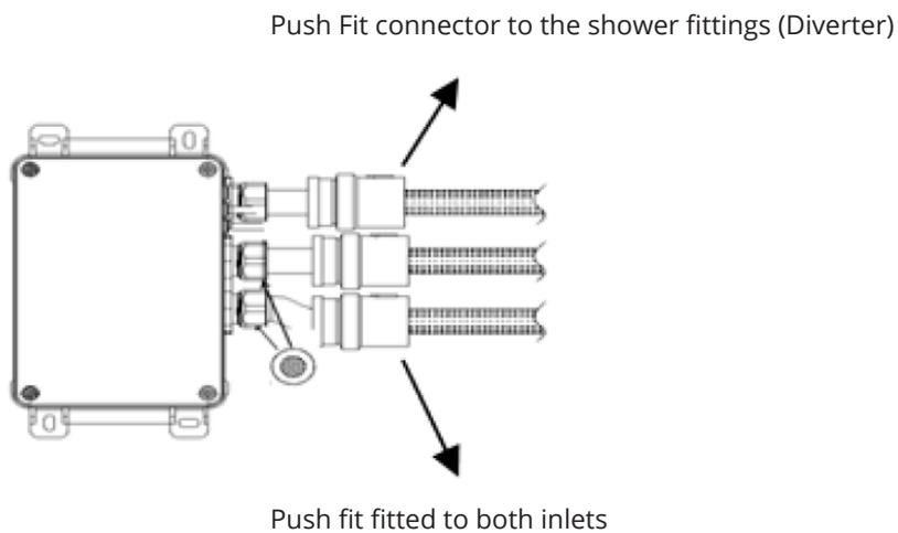
**NOTE:** Flush out the hot and cold supply pipes for 5 minutes minimum before connecting.
