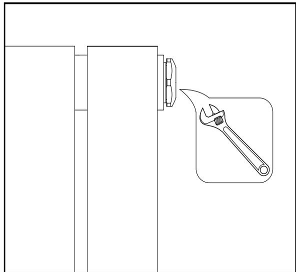
Please take care not to over tighten the bleed valve and blanking plug as this may damage the thread and/or the rubber O ring, which can result in damage to the radiator finish and leaking if not done correctly.
