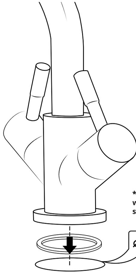
\*Remember to install the 'O' ring o washer between the mixer body & sanitary ware\*
