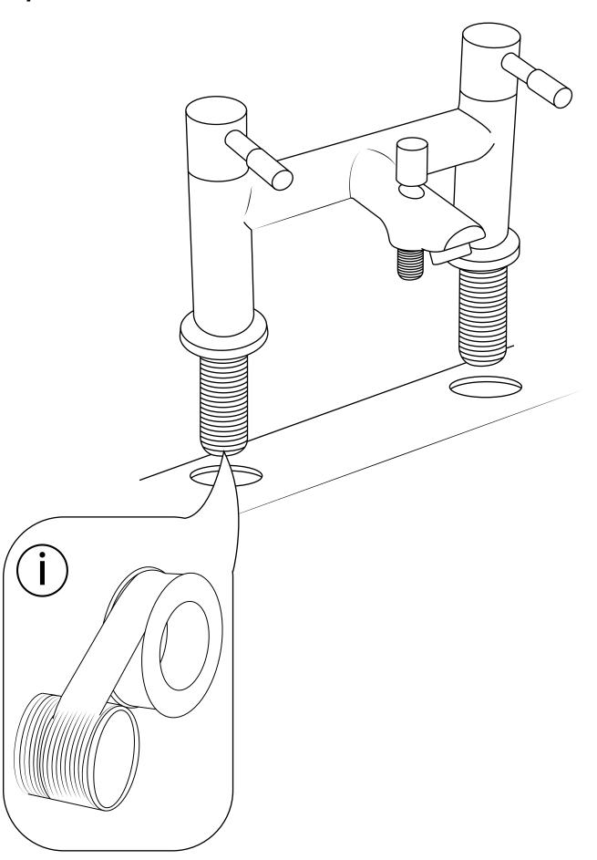
\*Remember to install the 'O' ring o washer between the mixer body & sanitary ware\*
